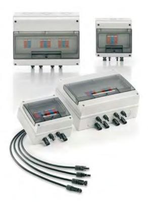
Lightning poses a risk to photovoltaic systems that generate renewable energy because of their large surface areas and exposure to the elements. Damage can affect individual areas or cause the entire system to fail. To protect all devices, the energy supply lines need to be equipped with surge protection in accordance with IEC 60364-7-712.
