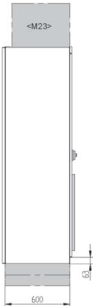
Dimension drawing 12: 380v~415V 315KW~355KW Line and motor connection from below
